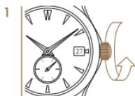
*Manually wind the movement by rotating the crown at least 30 times in the clockwise direction.*
